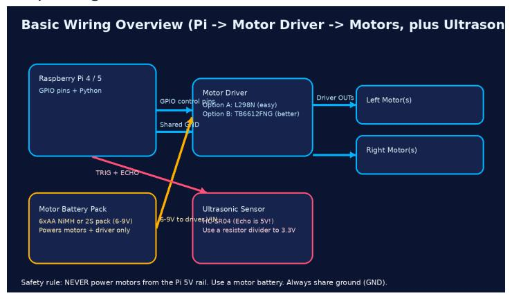
Your exact pin numbers can be changed, but keep them consistent in your code. The important parts are: shared ground (GND) and separate motor power.
